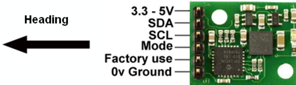
To enter the I2C mode of operation leave the mode pin unconnected
